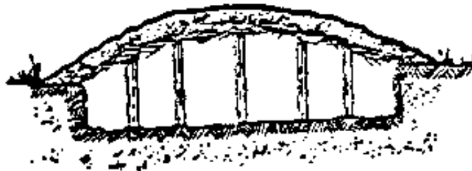
Fig. 40 Semi-subterranean potato storage house
