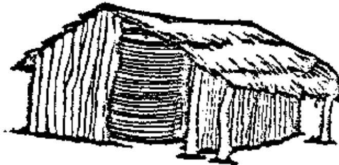
Fig. 57 Metal grain tank with thatch roof, Swaziland
