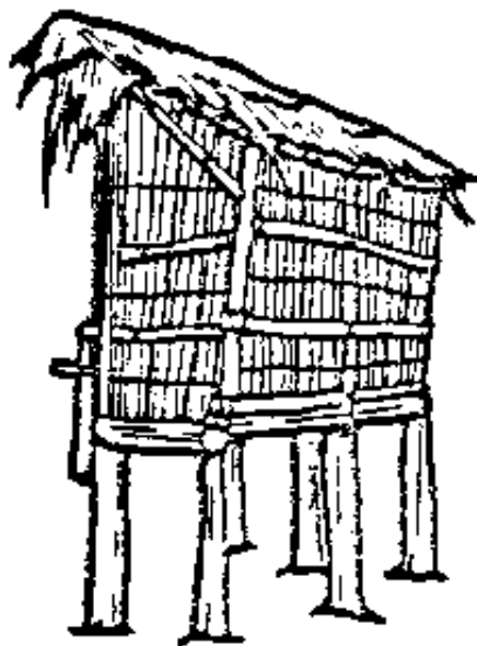
Fig. 41 Improved maize crib built from local materials
