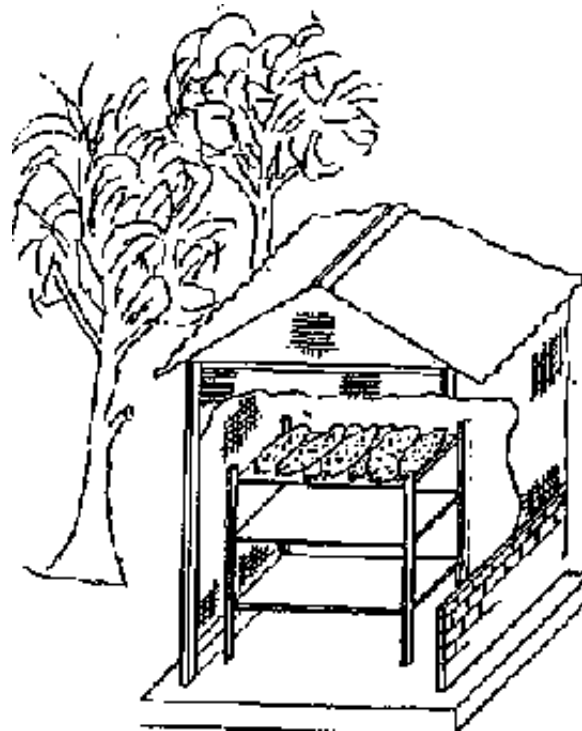
Fig. 13: Model of an improved yam barn with protective roof and walls (Source: NWANKITI and MAKURDI, 1989 (modified))
