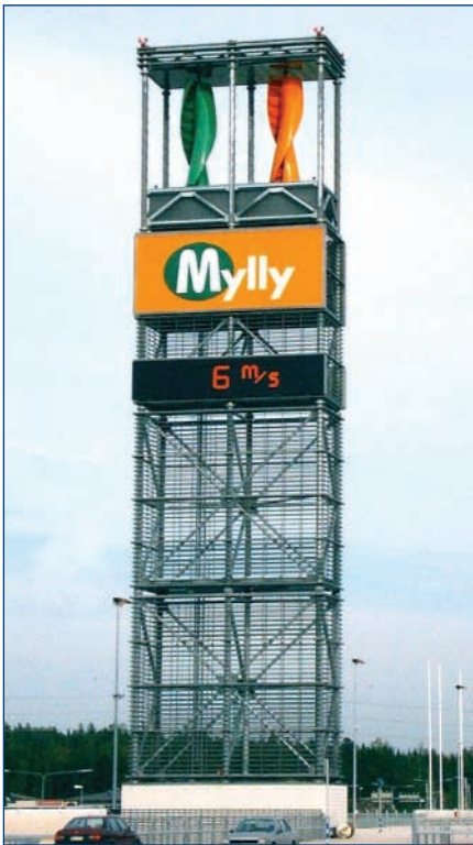
Figure 5: Twin 25 kW Windside-rotors powering a common 50 kW generator for heating use at Raisio shopping centre near Turku in Finland (Photograph from Oy Windside Production Ltd. Finland)
