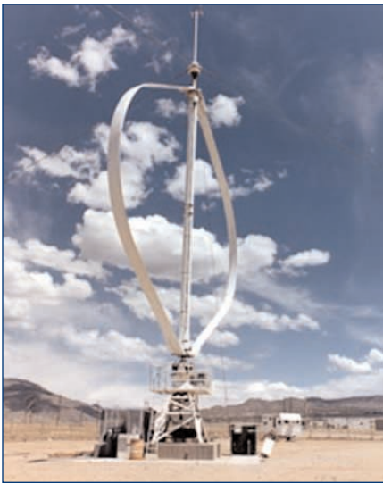
Figure 2: An example of a Darrieus wind turbine. This is a 60kW model at a test site at Sandia Laboratories (Photo: US Department of Energy)
