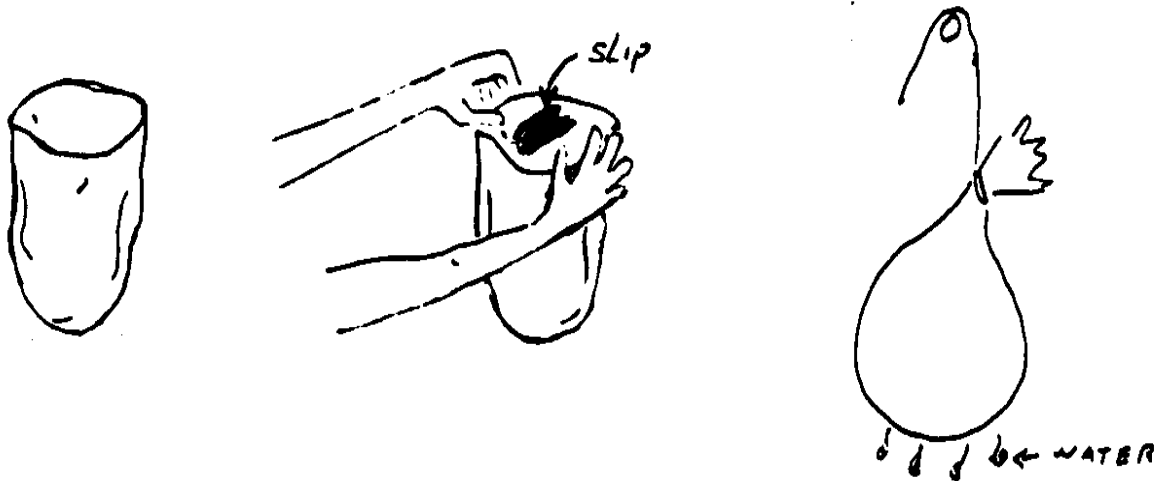
Figure 20. Drying Clay in a Cloth Bag
