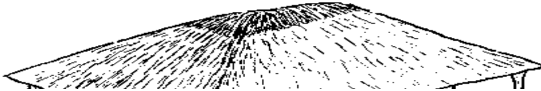
Wide thatch to keep rain and sun off the mud crib.
