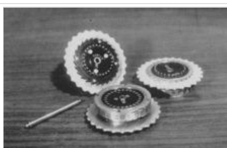
Three Enigma rotors and the shaft on which they are placed when in use.
