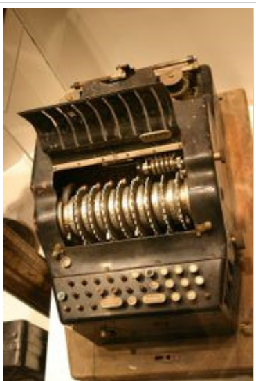
A rare 8-rotor printing Enigma.
