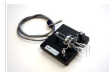
A commercially manufactured iambic paddle used in conjunction with an electronic keyer to generate high-speed Morse code, the timing of which is controlled by the electronic keyer. Manipulation of dual-lever paddles is similar to the Vibroplex, but pressing the right paddle generates a series of dahs , and squeezing the paddles produces dit-dah-dit-dah sequence. The actions are reversed for left-handed operators.
