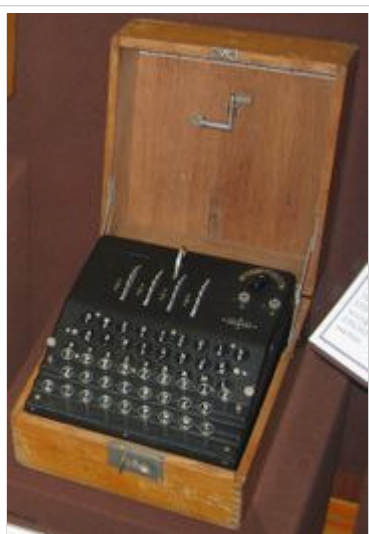
Enigma G, used by the Abwehr, had four rotors, no plugboard, and multiple notches on the rotors.
