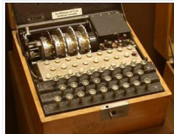
An Enigma model T (Tirpitz)—a modified commercial Enigma K manufactured for use by the Japanese.
