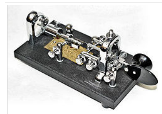
Vibroplex semiautomatic key. The paddle, when pressed to the right by the thumb, generates a series of dits , the length and timing of which are controlled by a sliding weight toward the rear of the unit. When pressed to the left by the knuckle of the index finger, the paddle generates a dah , the length of which is controlled by the operator. Multiple dahs require multiple presses. Left-handed operators use a key built as a mirror image of this one.
