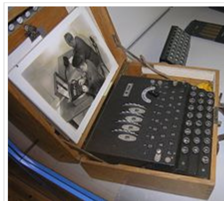
The four-wheel Swiss Enigma K, made in Germany, used re-wired rotors.
