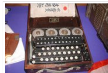
A Japanese Enigma clone, codenamed GREEN by American cryptographers.
