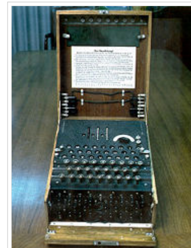
The plugboard, keyboard, lamps, and finger-wheels of the rotors emerging from the inner lid of a three-rotor German military Enigma machine
