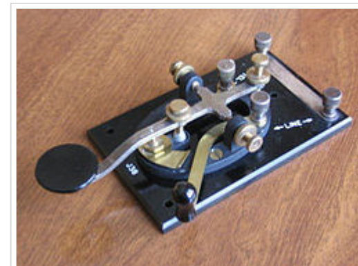
A typical "straight key." This U.S. model, known as the J-38, was manufactured in huge quantities during World War II, and remains in widespread use today. In a straight key, the signal is "on" when the knob is pressed, and "off" when it is released. Length and timing of the dits and dahs are entirely controlled by the operator.
