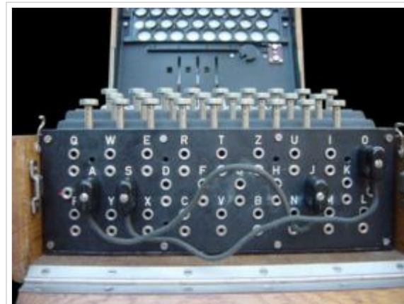
The plugboard ( Steckerbrett ) was positioned at the front of the machine, below the keys. When in use, there were up to 13 connections. In the above photograph, two pairs of letters have been swapped (S-O and J-A).
