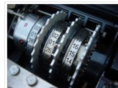
The Enigma rotor assembly. The three movable rotors are sandwiched between two fixed wheels: the entry wheel on the right and the reflector (here marked "B") on the left.
