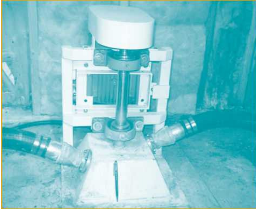
Figure 26. A double-jet Turgo induction generator system, 5-kW rated
