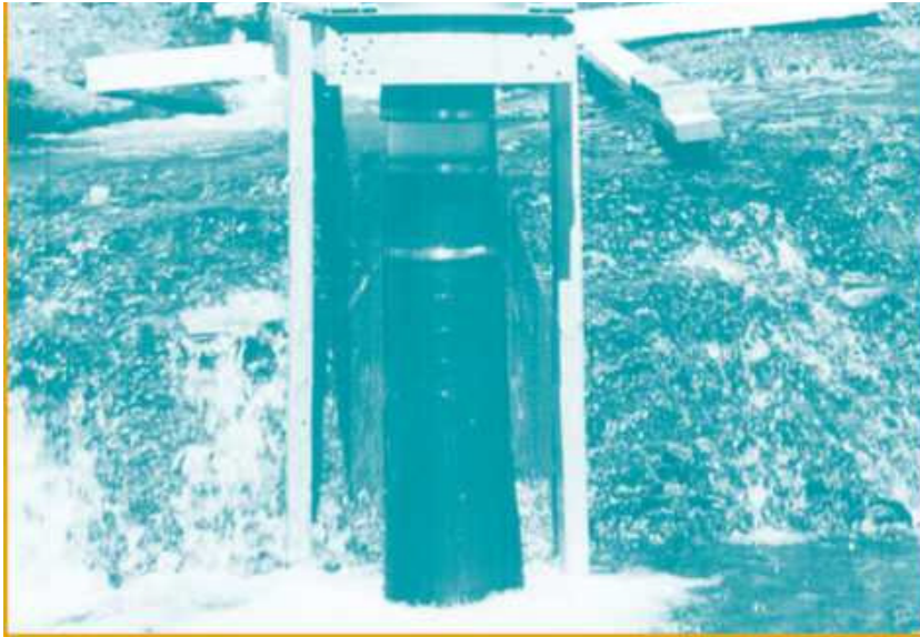
Figure 23. A 1-kW rated low-head battery-based system (photo courtesy of Energy Systems & Design)
