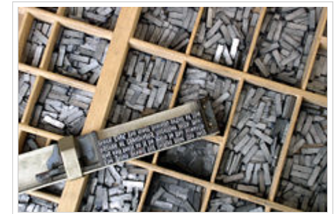
Movable metal type, and composing stick, descended from Gutenberg's press
