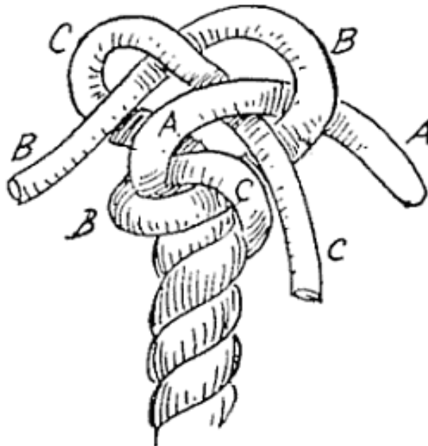
FIG. 124.—Wall crowned (making).
