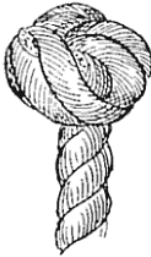
FIG. 123.—Double wall (complete).
