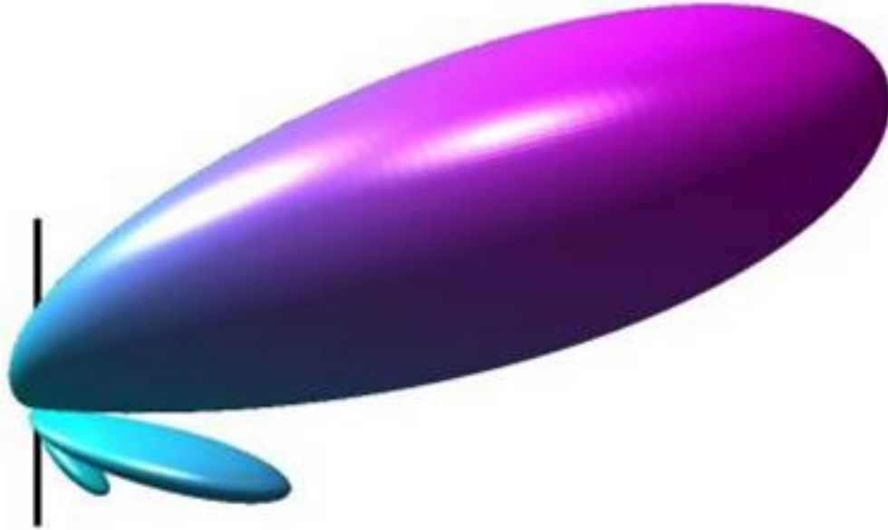
Figure 2.1: Visualization of a Beamformer
