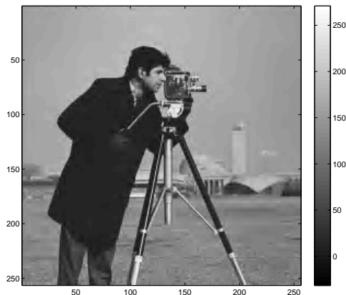
Figure 8.1: Compressive sensing reconstruction of the nonlinear approximation Cameraman image from Figure 5.2(b). Using M = 16384 random measurements of the K -term nonlinear approximation image (where K = 4096 ), we solve an \ell_1 -minimization problem to obtain the reconstruction shown above. The MSE with respect to the measured image is 0.08, so the reconstruction is virtually perfect.
