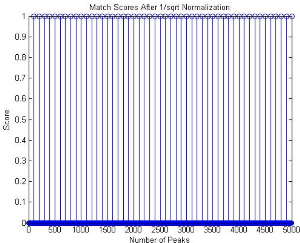
Figure 1.6: The same plot shown before, but with the square root dependency on number of peaks removed
