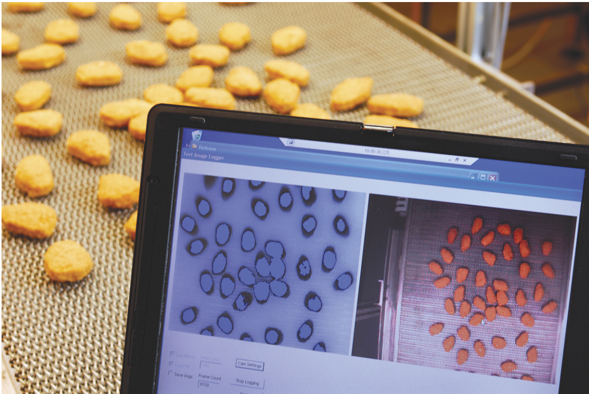
Figure 5.3: Monitoring heat distribution in chicken nuggets as they cook ensures quality, bacteria-free meat will emerge at the end of a conveyor belt oven [6].
