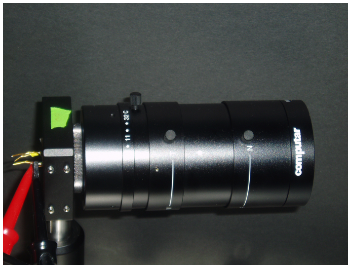
Figure 3.2: 10x zoom lens with photodiode mounted at focal point
