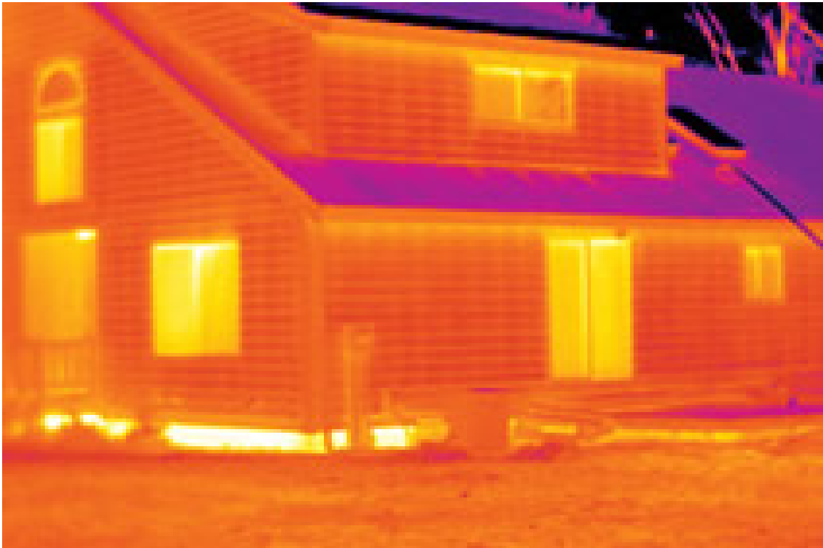
Figure 5.4: Energy audit of a home, showing areas where the house fails to retain heat [7].
