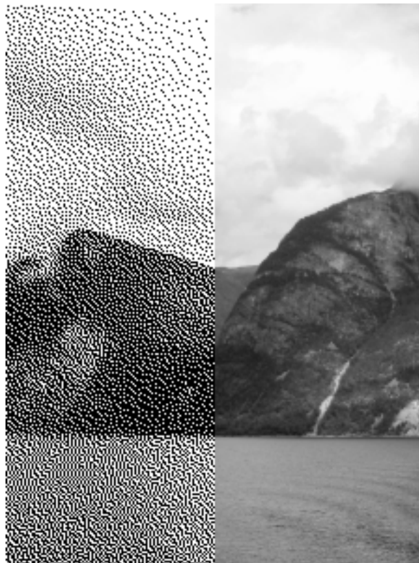
Figure 3.5: Mirror flickering on a DMD creates the illusion of grayscale through PWM [11]
