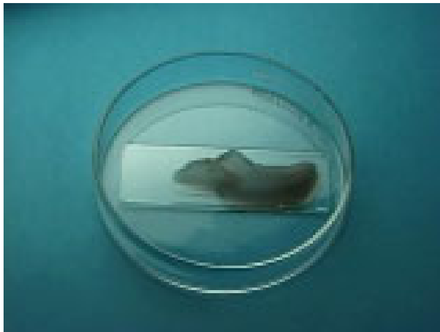
Figure 2.23: Image of the preparation of the silver layer seen as a dark precipitate.
