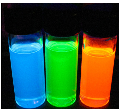
Figure 2.20: Picture of cadmium selenide (CdSe) quantum dots, dissolved in toluene, fluorescing brightly, as they are exposed to an ultraviolet lamp, in three noticeable different colors (blue \sim 481 nm, green \sim 520 nm, and orange \sim 612 nm) due to the quantum dots' bandgap (and thus the wavelength of emitted light) depends strongly on the particle size; the smaller the dot, the shorter the emitted wavelength of light. The "blue" quantum dots have the smallest particle size, the "green" dots are slightly larger, and the "orange" dots are the largest.
