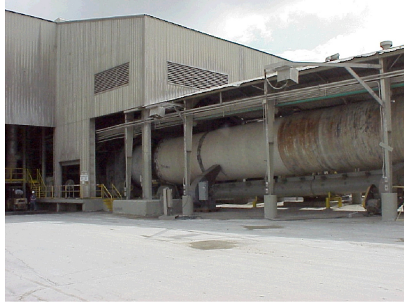
Figure 4.10: A wet rotary kiln (Copyright Halliburton Energy Services).
