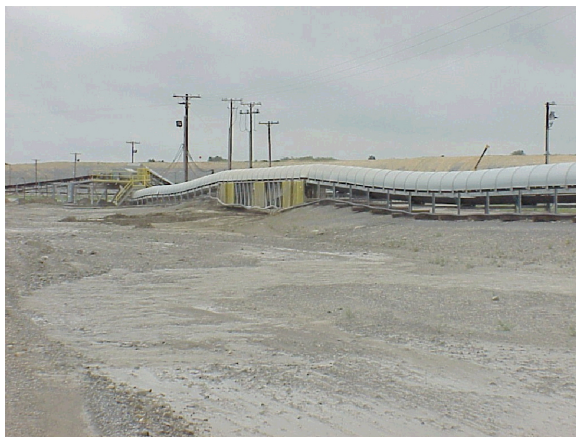
Figure 4.4: Covered conveyor belt for limestone transport (Copyright Halliburton Energy Services).
