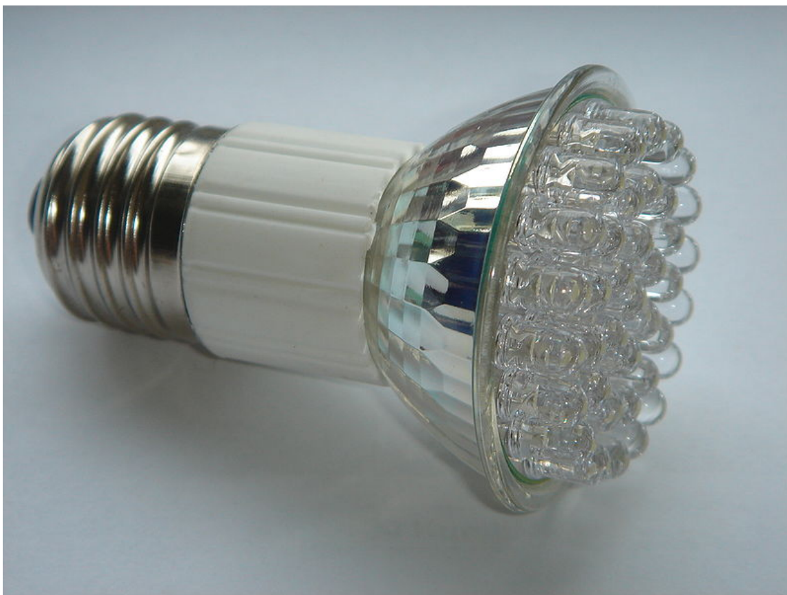
Figure 8.58: Solid State Lighting (SSL) Solid state lighting (SSL) is comprised of many small LEDs. Since they release very little energy as heat, they are cool to the touch and highly efficient. Source: Ocrho 168
