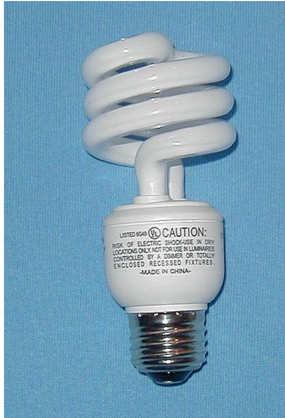
Figure 8.57: Compact Fluorescent Light Bulb Over its lifetime, each standard (13 watt) CFL will reduce electricity bills by about $30 and emissions from 200 lbs of coal over its lifetime. Source: Kevin Rector 165
