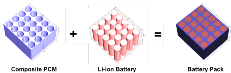
Figure 8.75: Application with PCM Technology. A pack of Li-ion batteries kept at a narrow temperature range with a proper use of passive thermal management system. Source: AllCell's PCM Technology©
