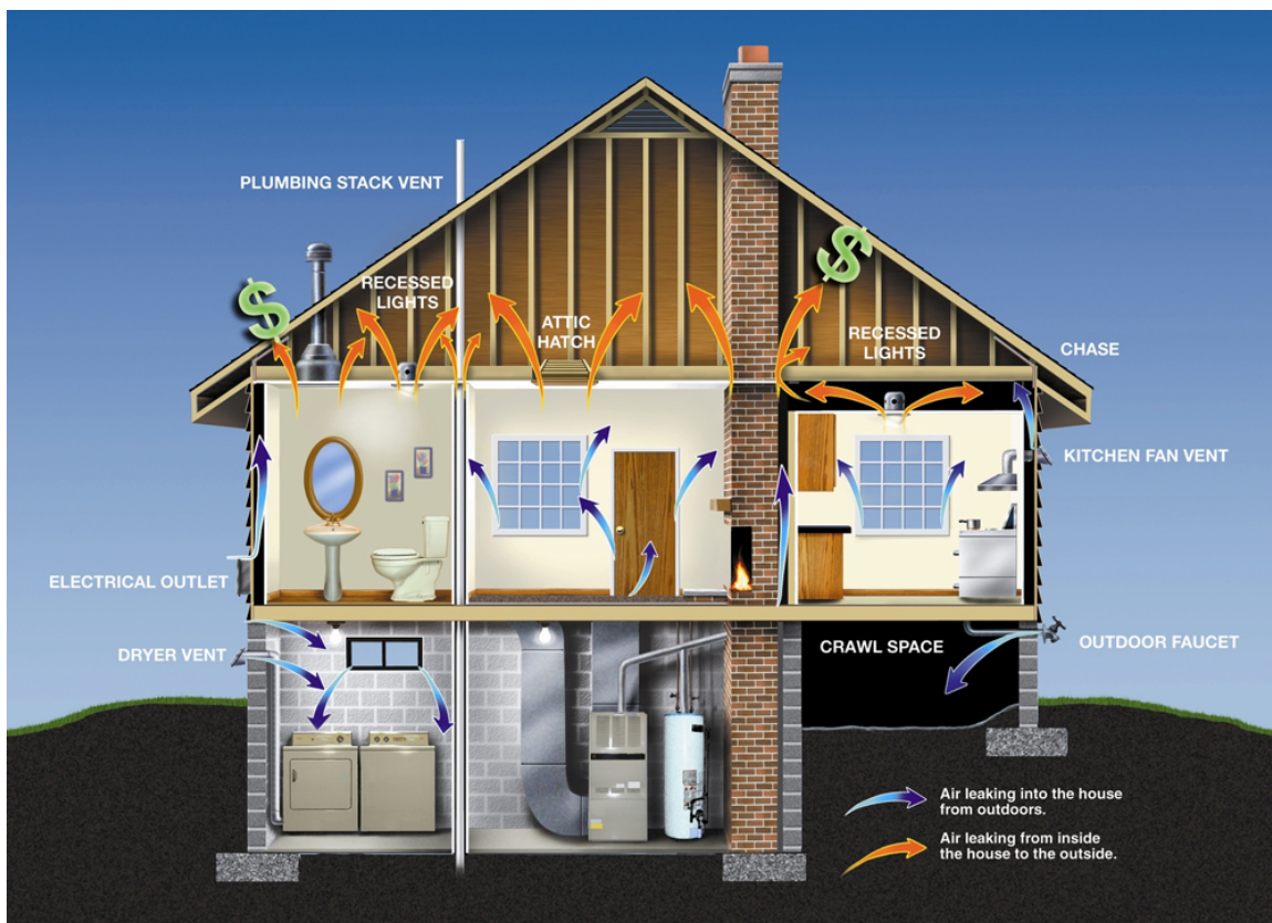
Figure 8.60: Diagram of a Leaky Home Diagram shows the various points in a home where energy may leak. Source: ENERGY STAR 171
