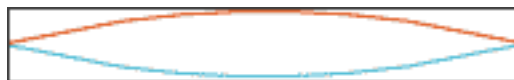
Figure 1.7: The standing waves inside the tube represent back-and-forth motion of the air. Since the air can't move through the end of the tube, a closed tube must have a node at each end, just like a string held at both ends.
