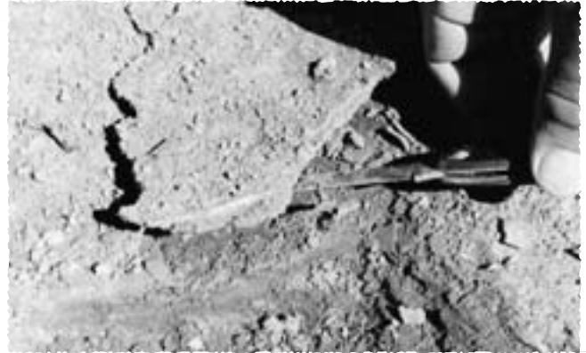
A thin surface crust caused by raindrop impact on a bare soil with poor structure. Photo: T.F. Shaxson.
