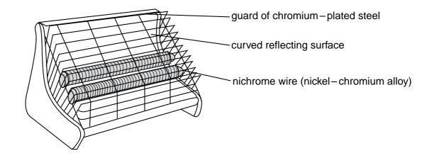
Which method would be used to plate the chromium on to the steel?
