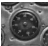
Manifold pressure gauge
