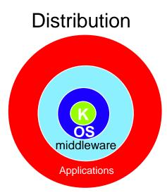
Linux Kernel + Operating System + Middleware + Applications = Distribution IBM will not distribute Linux software itself, but will provide support in OS/400 for the Linux applications.
