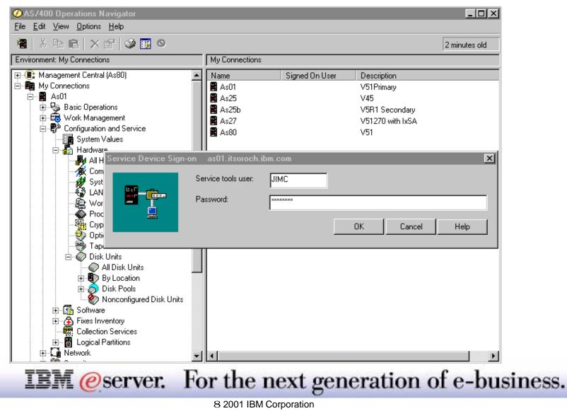
Presuming Application Administration has specified Disk Units can be managed and your workstation has Configuration and Service installed, you see "Disk Units" branch at the bottom of the Configuration and Service-Hardware tree structure.
