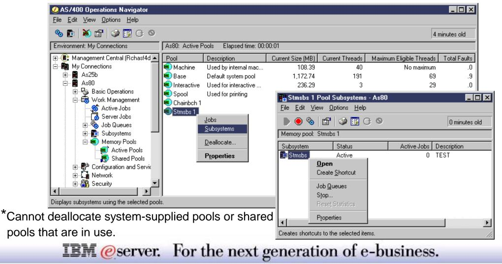
The Active Pools container contains all shared and private memory pools that are currently in use. In essence, an active pool means that main storage has been allocated to it. The information displayed in the right pane is similar to what you typically see at the bottom of the WRKSYSSTS display. The list of active pools is shown in the following predefined order by default:
