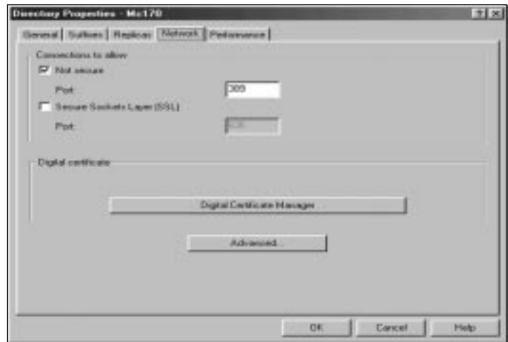
Figure 5: The Directory Server properties allow you to configure SSL and specify a server where your LDAP data is replicated, as well as some other configuration functions.
