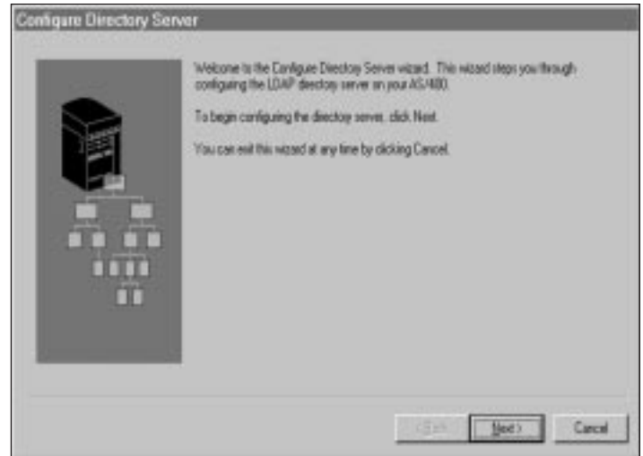
Figure 4: The OpsNav Configure Directory wizard is the only place where you can configure your AS/400 LDAP Directory server.
