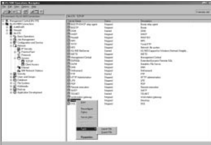
Figure 3: You perform most of the LDAP configuration tasks from the AS/400 Directory pop-up context menu.
