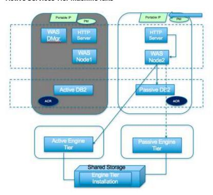
Failure: The machine in dark grey colour has failed all the communication to that machine is stopped.
