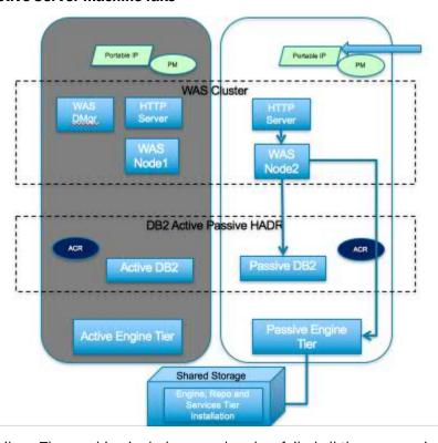
Failure: The machine in dark grey colour has failed all the communication to that machine is stopped.
