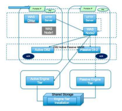
Failure: The WebSphere node, Node 1 shown in dark grey colour goes away, and all the connections between this and other processes are broken.
