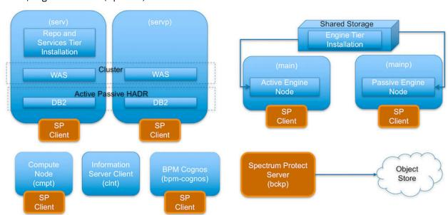
Spectrum Protect server software is installed in the Spectrum Protect server machine and the Spectrum Protect Client software is installed in the rest except the IIS Windows Client machine.
