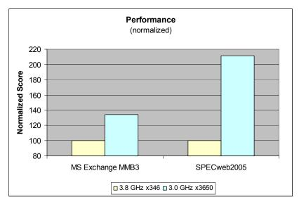
**Figure 2.** *Performance comparison of x346 and x3650*
