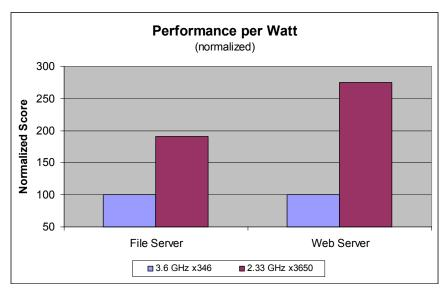
Figure 3. Performance-per-watt comparison of IBM servers using SC and DC Intel processors
