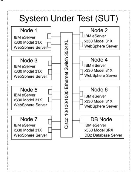
Figure 7.3.1: System Under Test
