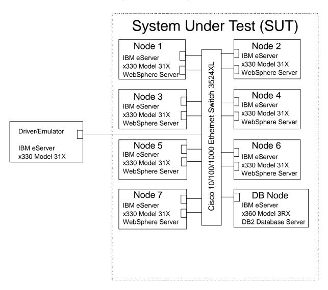
10/100/1000Mbit switch. The DB node (xSeries 360) was connected with a 1Gb adapter to this switch.
