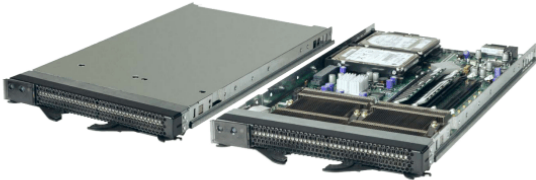
Figure 11. View of an HS20 Blade Server
