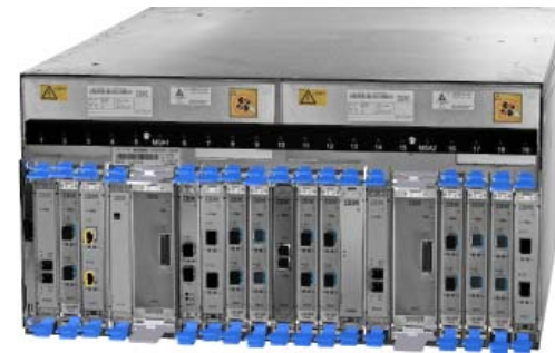
PCIe I/O drawer 32 I/O slots
