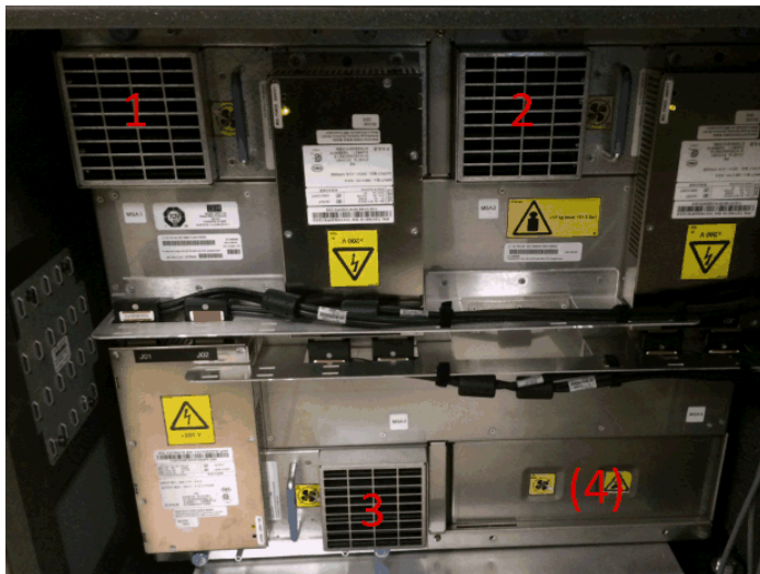
Rear View of 2 CPC Drawer System with 3 Blowers Installed
