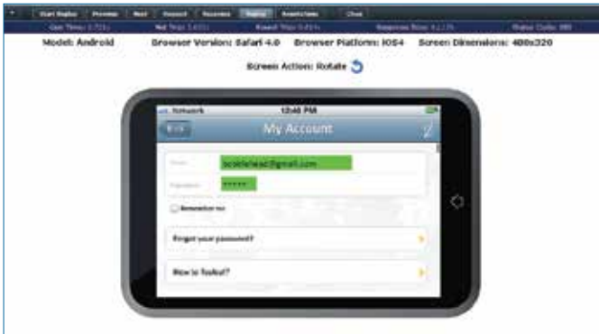
Figure 1: Enhanced mobile Web session replay helps users see orientation-specific actions like device rotation (i.e., portrait or landscape).
