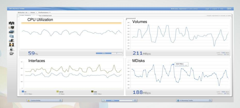
Gathers system level performance statistics (CPU utilization; port utilization and I/O rates; volume and MDisk I/O rate, bandwidth, latency) in real time with sampling rates down to 5 sec.
