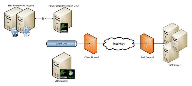
In this setup, ESA connects through your internet connection by the default route. For this type of configuration, you can optionally use a second network card to physically separate the local system network from the internet enabled network.
