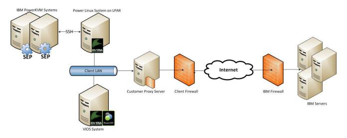
To forward ESA packets, the proxy server must support the basic proxy header functions (as described in RFC #2616) and the CONNECT method. Optionally, basic proxy authentication (RFC #2617) may be configured so that the ESA authenticates before attempting to forward packets through your proxy server.
