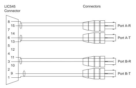
Figure 2-119. LIC545 Cable Pin Assignment
