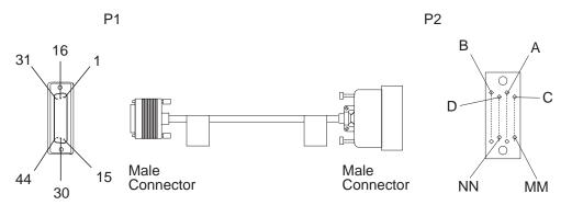
Figure 2-59. V.35 Cable: LIC512 to DCE
