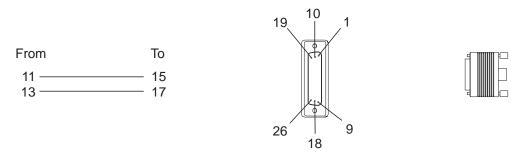
Figure 2-123. LIC546 Wrap Plug Pin Assignments
