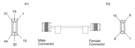
Figure 2-96. X.21 Cable: LIC522 to DTE
