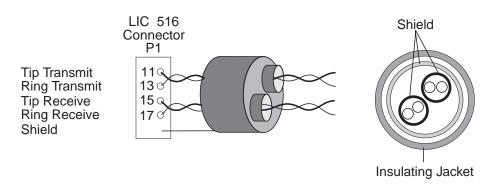
Figure 2-82. LIC516 E1 Cable Pin Assignment
