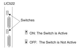
Figure 2-102. LIC522 Switches on Front Module
