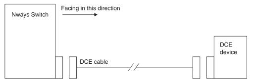
The DCE cable goes from the Nways Switch to a DCE device.
