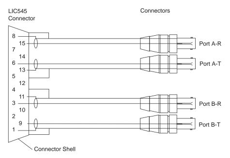
Figure 2-118. LIC545 IBM Cable Pin Assignment
