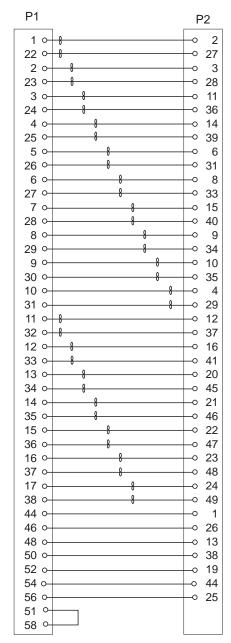
Figure 2-110. HSSI Cable: LIC530-to-DCE Pin Assignment
