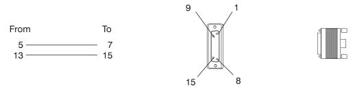
Figure 2-83. LIC517 Wrap Plug Pin Assignment
