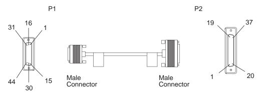
Figure 2-94. V.36 Cable: LIC522 to DCE
