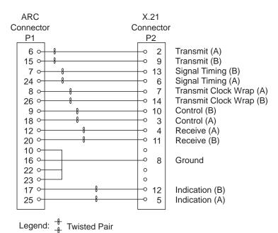
Figure 2-48. X.21 Cable: ARC-to-DCE Pin Assignment
