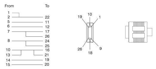
Figure 2-37. ARC V.35 Wrap Plug Pin Assignment (Part Number 80G3743)
