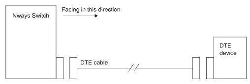
The DTE cable goes from the Nways Switch to a DTE device.
