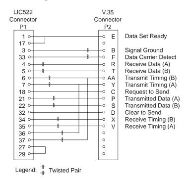
Figure 2-88. V.35 Cable: LIC522-to-DTE Pin Assignment for Cable Up to 30 meters (100 feet)
