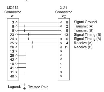
Figure 2-66. X.21 TRANSFIX Cable: LIC512 to DCE Pin Assignment
