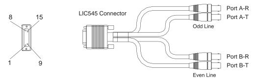
Figure 2-117. Cable (PN 80G2226) Provided with the LIC545 ( 4 Cables)
