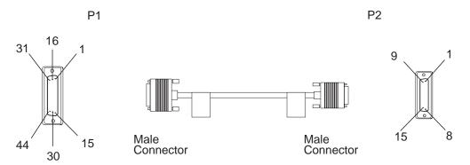
Figure 2-100. X.21 TRANSFIX Cable: LIC522 to DCE
