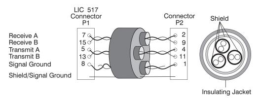
Figure 2-85. Cable: LIC517 to DCE Pin Assignment
