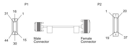
Figure 2-92. V.36 Cable: LIC522 to DTE
