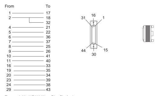
Figure 2-86. LIC522 Wrap Plug Pin Assignment
