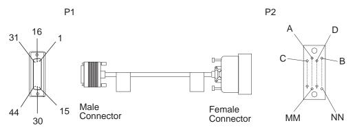
Figure 2-87. V.35 Cable: LIC522 to DTE
