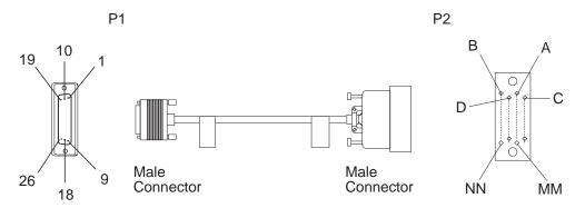
Figure 2-43. V.35 Cable: ARC to DCE
