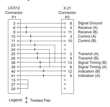
Figure 2-62. X.21 Cable: LIC512 to DTE Pin Assignment
