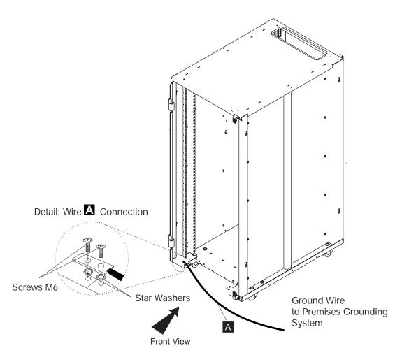
Figure 2-20. Grounding of the 2220-500 to the Premises Grounding System in a 29 U Rack
