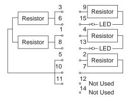
Figure 2-31. LIC511 Wrap Plug Pin Assignment
