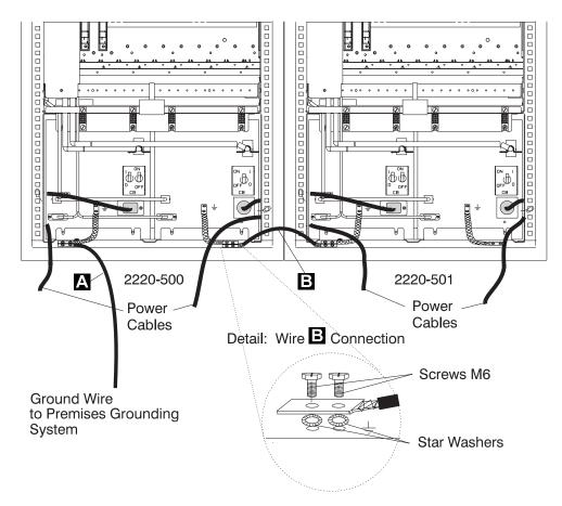
Figure 2-23. Grounding Connection Between the 2220-500 and the 2220-501
