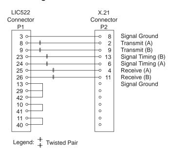
Figure 2-101. X.21 TRANSFIX Cable: LIC522-to-DCE Pin Assignment
