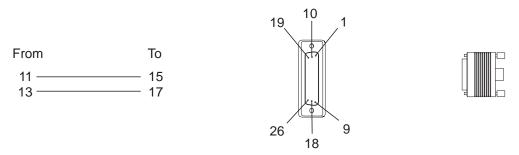
Figure 2-113. LIC544 Wrap Plug Pin Assignment
