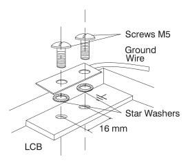
Figure 2-27. Bellcore Specification Connection
