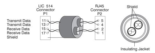
Figure 2-74. LIC514 RJ-45 J1 Cable Pin Assignment
