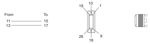
Figure 2-144. LIC567 Wrap Plug Assignment
