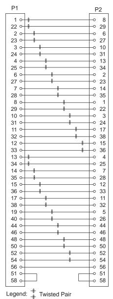
Figure 2-112. HSSI Cable: LIC530-to-LIC530 DCE/DTE Pin Assignement
