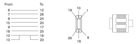
Figure 2-38. ARC X.21 Wrap Plug Pin Assignment (Part Number 80G3744)
