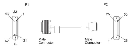
Figure 2-107. HSSI Cable: LIC530 to DTE
