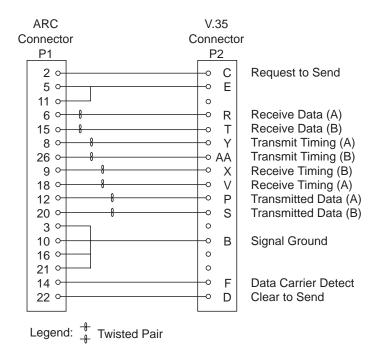
Figure 2-46. V.35 Cable: ARC-to-DTE Pin Assignment
