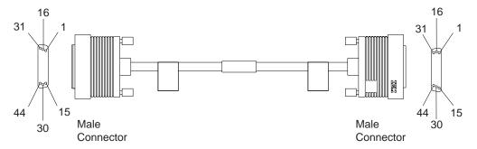
Figure 2-34. LCBB-to-LCBE Cable. This cable is 35 cm (1.15 feet) long.
