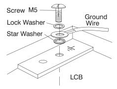
Figure 2-26. Standard Connection
