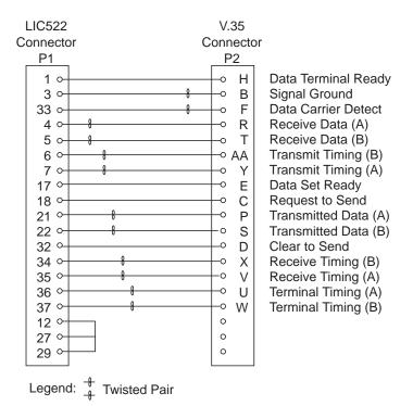
Figure 2-89. V.35 Cable: LIC522-to-DTE Pin Assignment for Cables Longer than 30 meters (100 feet)
