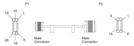
Figure 2-47. X.21 Cable: ARC to DCE
