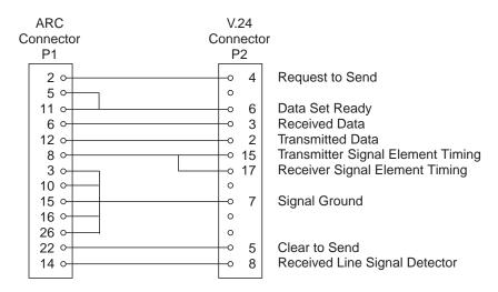
Figure 2-42. V.24 Cable: ARC-to-DTE Pin Assignment
