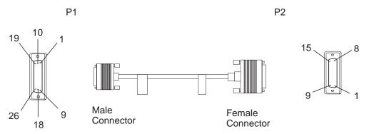
Figure 2-49. X.21 Cable: ARC to DTE
