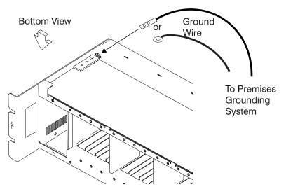
Figure 2-25. LCB Grounding Using Ground Wire
