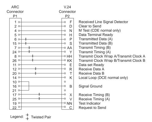
Figure 2-44. V.35 Cable: ARC-to-DCE Pin Assignment
