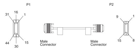
Figure 2-63. X.21 Cable: LIC512 to DCE
