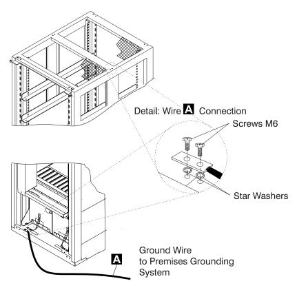
Figure 2-19. Grounding of the 2220-500 to the Premises Grounding System in a 37 U Rack
