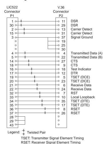
Figure 2-95. V.36 Cable: LIC522-to-DCE Pin Assignment
