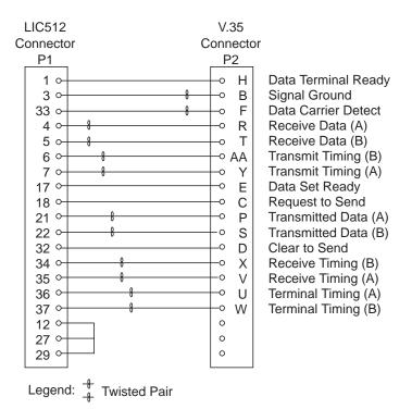
Figure 2-58. V.35 Cable: LIC512 to DTE Pin Assignment for Cable Longer than 30 meters (100 feet)
