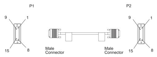
Figure 2-84. Cable: LIC517 to DCE
