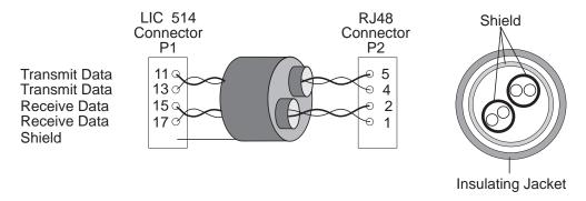
Figure 2-73. LIC514 RJ-48 T1 Cable Pin Assignment
