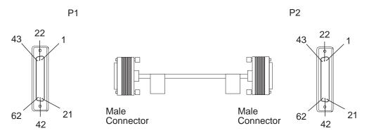
Figure 2-111. HSSI Cable: LIC530 to LIC530 DCE/DTE
