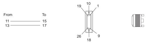
Figure 2-80. LIC516 Wrap Plug Pin Assignment
