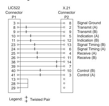
Figure 2-99. X.21 Cable: LIC522-to-DCE Pin Assignment
