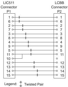
Figure 2-32. Interchange Circuits for LIC511 Attachment Cables
