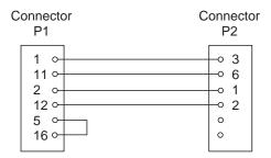
Figure 2-11. Cable Pin Assignment
