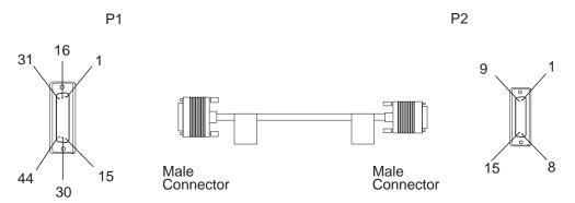
Figure 2-98. X.21 Cable: LIC522 to DCE
