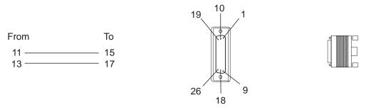
Figure 2-71. LIC514 Wrap Plug Pin Assignment
