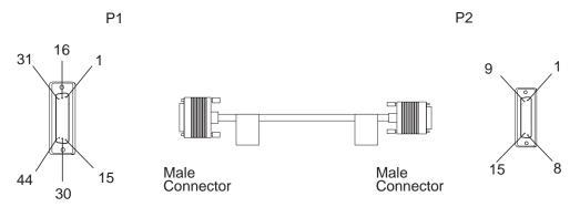
Figure 2-65. X.21 TRANSFIX Cable: LIC512 to DCE
