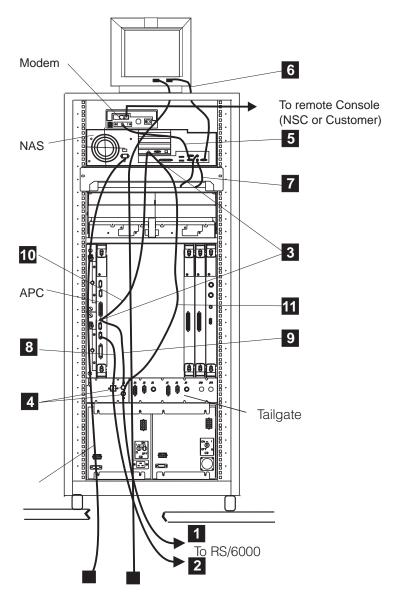
Figure 2-1. Nways Switch Administration Station Cables (Here Installed in 29 U Rack)
