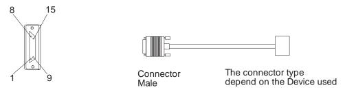
Figure 2-17. Cable for Connection to Tailgate Connectors J5 and J8
