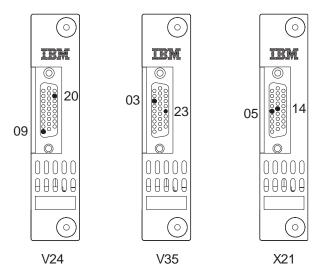
Figure 2-35. ARC Front Connector
