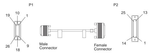
Figure 2-41. V.24 Cable: ARC to DTE
