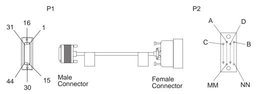
Figure 2-56. V.35 Cable: LIC512 to DTE
