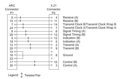
Figure 2-50. X.21 Cable: ARC-to-DTE Pin Assignment
