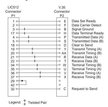
Figure 2-60. V.35 Cable: LIC512 to DCE Pin Assignment
