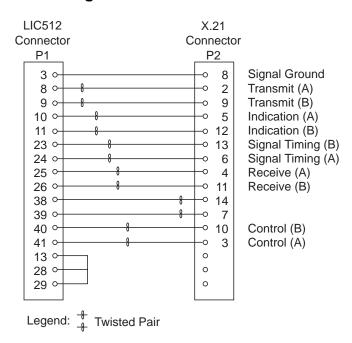
Figure 2-64. X.21 Cable: LIC512 to DCE Pin Assignment
