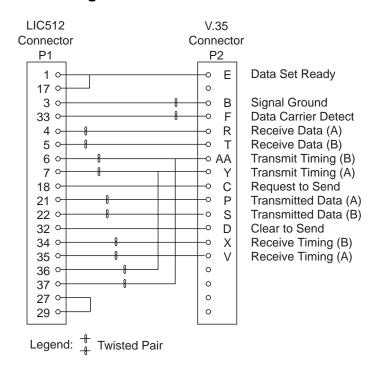
Figure 2-57. V.35 Cable: LIC512 to DTE Pin Assignment for Cable Up to 30 meters (100 feet)
