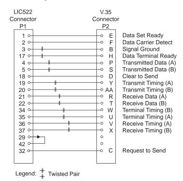
Figure 2-91. V.35 Cable: LIC522-to-DCE Pin Assignment
