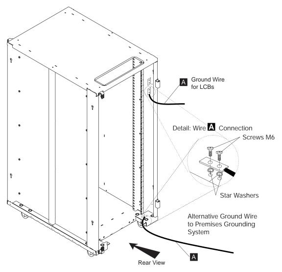
Figure 2-21. LCB and Alternative Ground Wire in 29 U Rack
