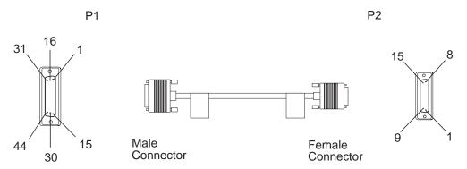
Figure 2-61. X.21 Cable: LIC512 to DTE
