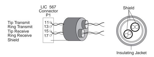
Figure 2-143. LIC563 E1 Cable Pin Assignment
