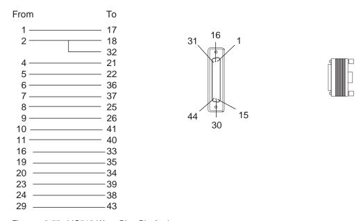
Figure 2-55. LIC512 Wrap Plug Pin Assignment
