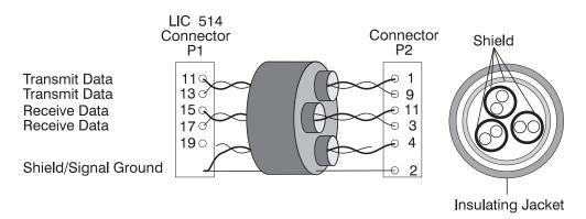
Figure 2-76. LIC514 DB15 Cable Pin Assignment
