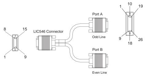
Figure 2-124. Y Cables (PN 80G2225) Provided with the LIC546
