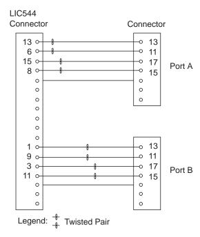
Figure 2-115. LIC544 Cable Pin Assignment
