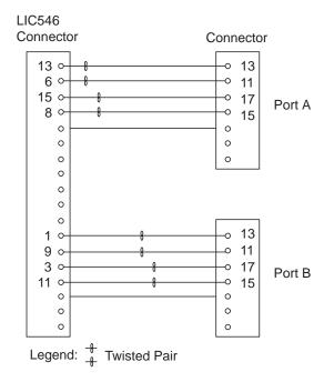
Figure 2-125. LIC546 Cable Pin Assignment
