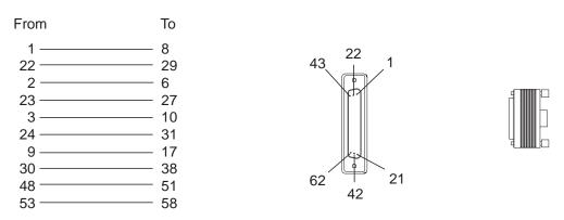
Figure 2-106. LIC530 Wrap Plug Pin Assignment
