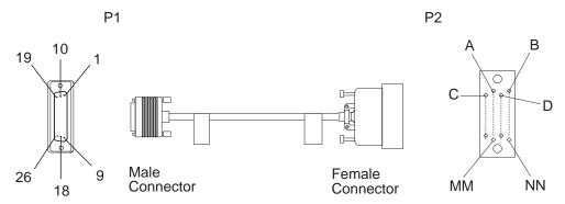
Figure 2-45. V.35 Cable: ARC to DTE
