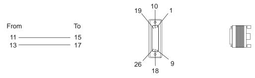
Figure 2-141. LIC563 Wrap Plug Assignment
