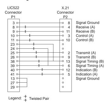
Figure 2-97. X.21 Cable: LIC522-to-DTE Pin Assignment
