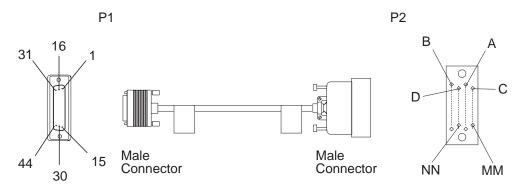
Figure 2-90. V.35 Cable: LIC522 to DCE
