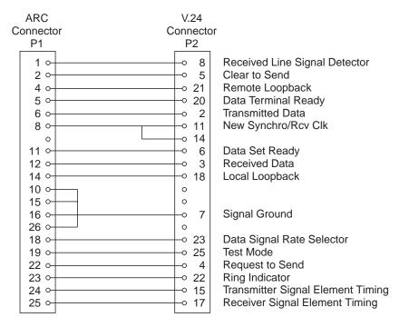
Figure 2-40. V.24 Cable: ARC-to-DCE Pin Assignment
