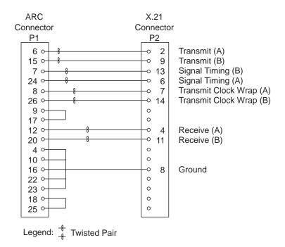
Figure 2-52. X.21 Cable: ARC to Transfix Pin Assignment
