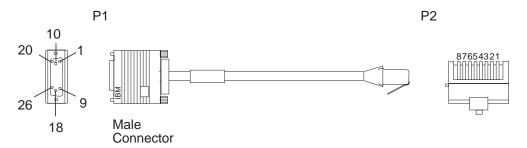
Figure 2-72. LIC514 RJ-48 T1 and J1 Cable
