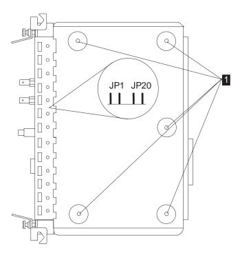
Figure 2-105. LIC523 Module Opening and Jumper Positions
