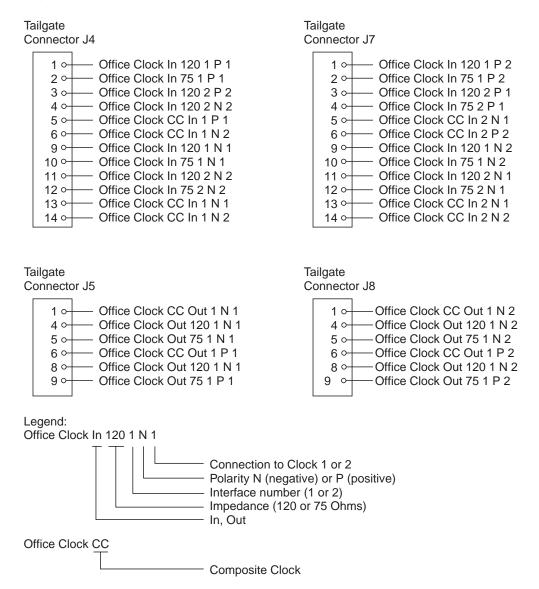
Figure 2-18. External Cable Pin Assignments (Between the 2220 Tailgate and the External Device)
