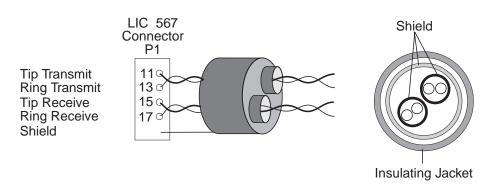
Figure 2-146. LIC567 E1 Cable Pin Assignment
