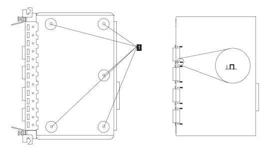
Figure 2-121. LIC545 Module Openning and Jumper Positions
