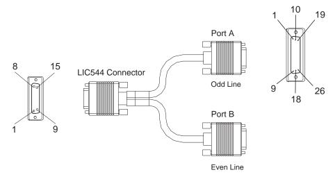
Figure 2-114. LIC544 Y Cable (PN 80G2225) for T1/J1 Connection ( 4 Cables)
