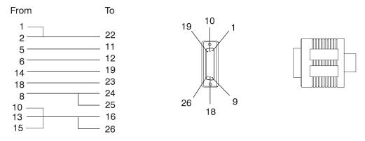
Figure 2-36. ARC V.24 Wrap Plug Pin Assignment (Part Number 80G3742)
