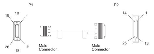
Figure 2-39. V.24 Cable: ARC to DCE
