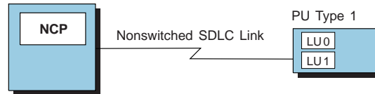
Figure 5-21. SDLC Devices Attached to Nonswitched Telecommunication Links
