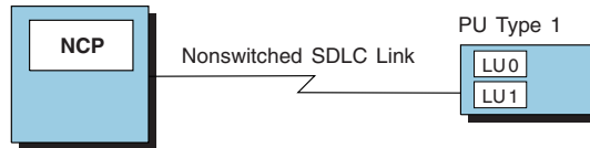
Figure 5-21. SDLC Devices Attached to Nonswitched Telecommunication Links
