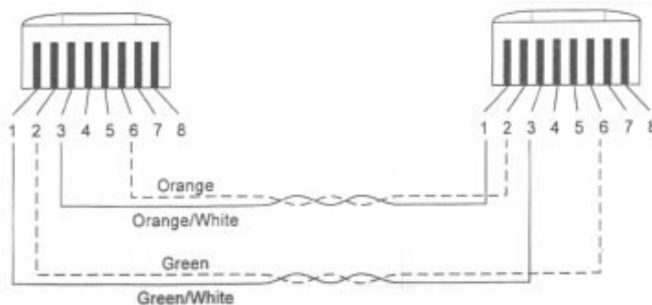
Figure B-4. Crossover UTP Cable (RJ-45 to RJ-45), T568-A
