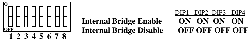
Figure 2-4 TX Module DIP Switch Setting
