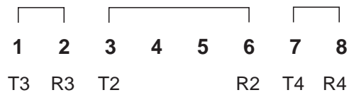
Figure 9. OPEN DECconnect Polarization
