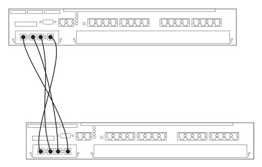
Figure 3-3. Cabling for the Optical Fiber RI/RO Module
