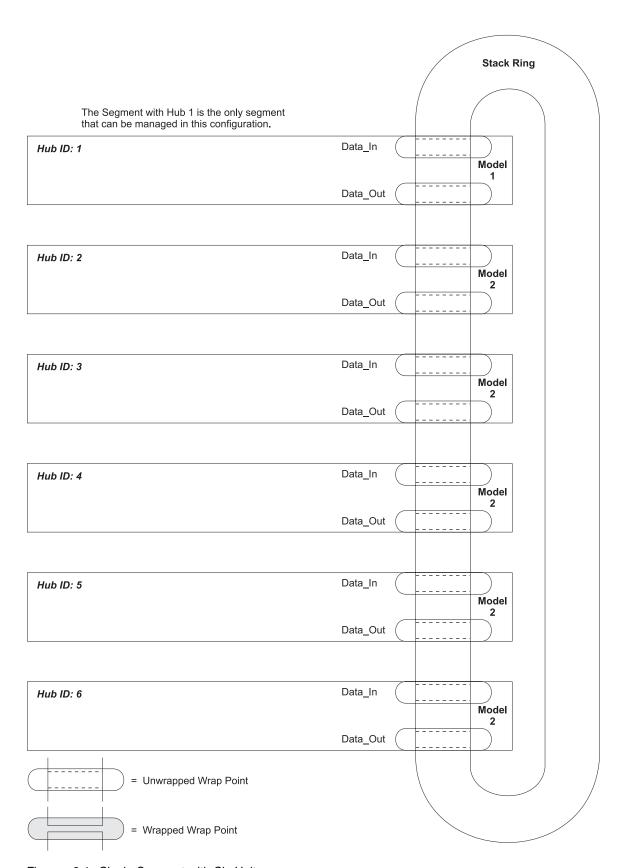
Figure 6-1. Single Segment with Six Units
