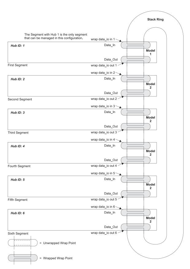
Figure 6-2. Six Units with Six Segments
