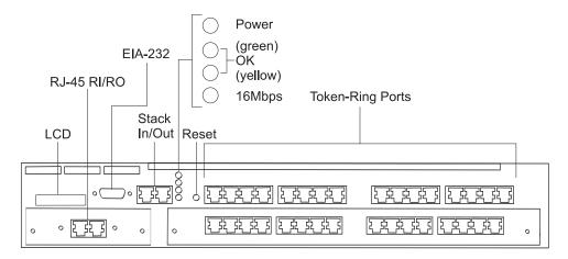
Figure 5-1. 8239 Model 1 LEDs and LCD
