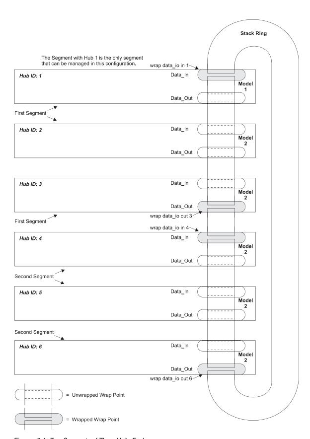
Figure 6-4. Two Segments of Three Units Each
