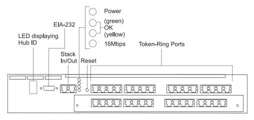
Figure 5-2. 8239 Model 2 LEDs
