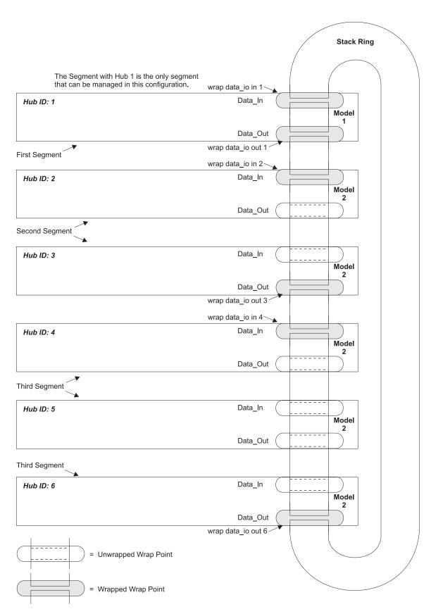
Figure 6-5. Six Units with Three Segments
