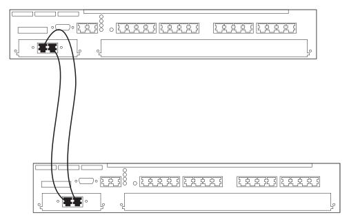
Figure 3-4. Cabling for the RJ-45 RI/RO Module
