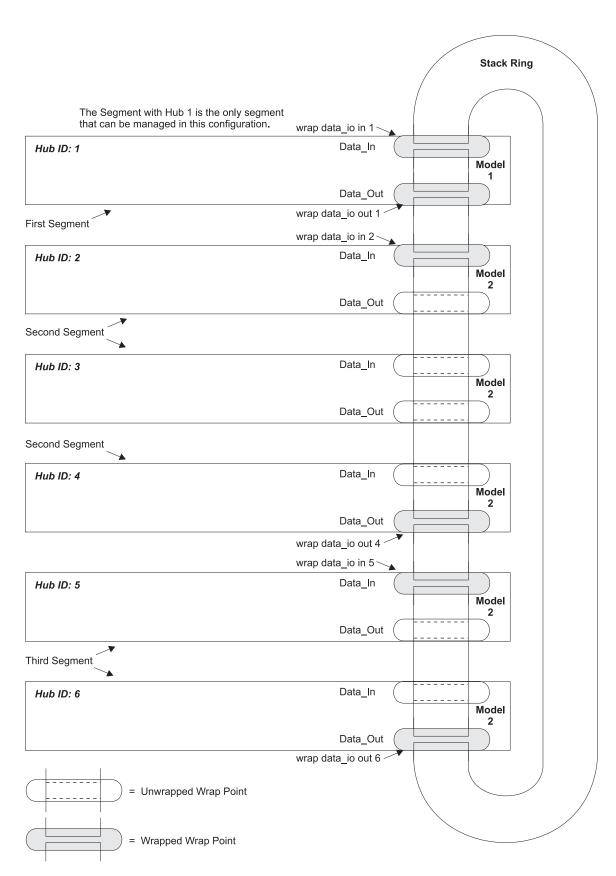
Figure 6-6. Six Units with Three Segments
