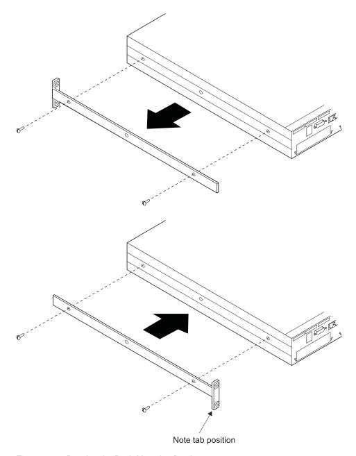
Figure 2-1. Rotating the Rack-Mounting Brackets
