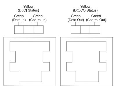
Figure 5-5. Stack In/Stack Out LEDs
