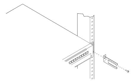
Figure 2-2. Attaching the Cable Management Bracket
