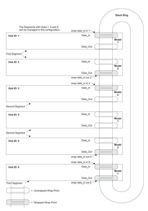
Figure 6-8. Six Units with Three Segments
