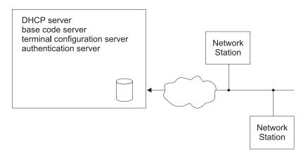
Figure 23. Remote Network Station without a Thin Server
