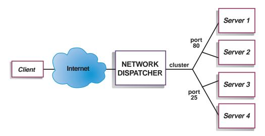
Figure 5. Example of Network Dispatcher Configured With a Single Cluster and 2 Ports
