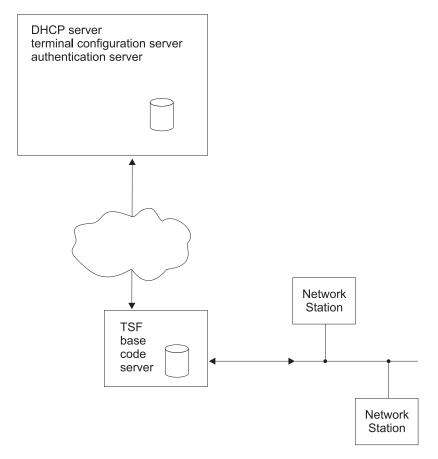
Figure 24. Remote Network Station with a Thin Server
