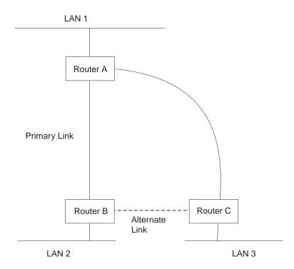
If the primary link between routers A and B fails, WAN reroute establishes an alternate link between routers B and C. Routers A and B can then communicate through router C.
