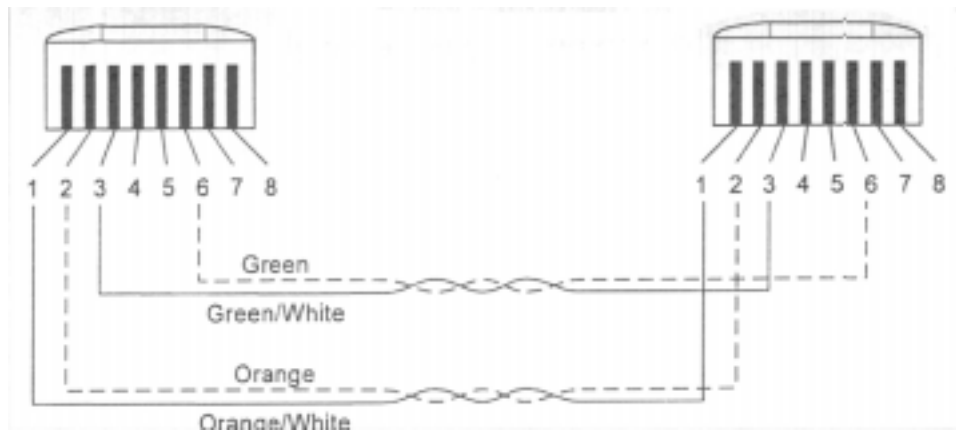
Figure B-2 Straight-Through UTP Cable (RJ-45 to RJ-45), T568B
