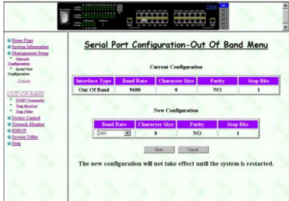
Figure 5-10 Serial Port Configuration-Out Of Band Menu
