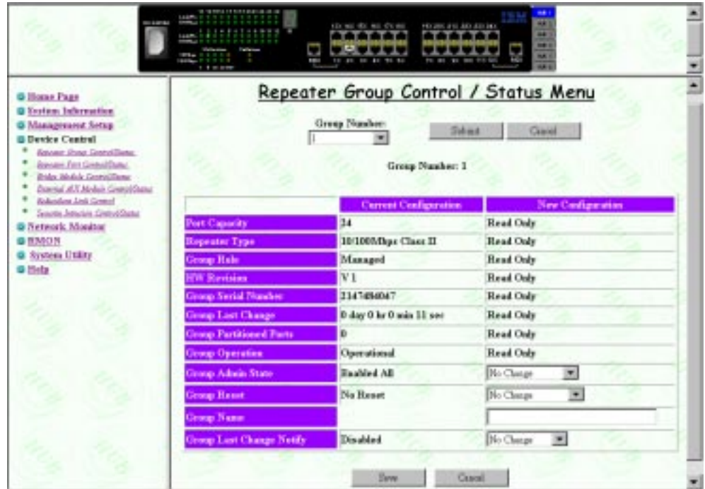
Figure 5-14 Repeater Group Control/Status Menu
