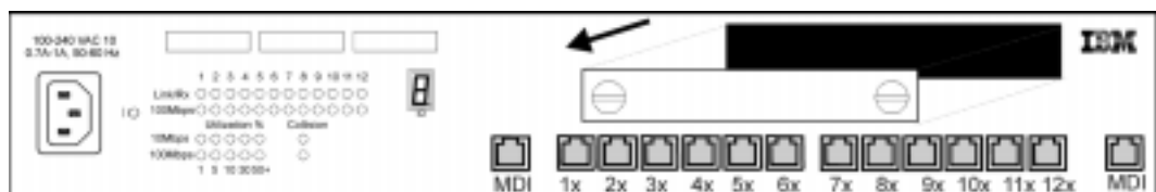
Figure 2-5 Removing the Blank Module Panel
