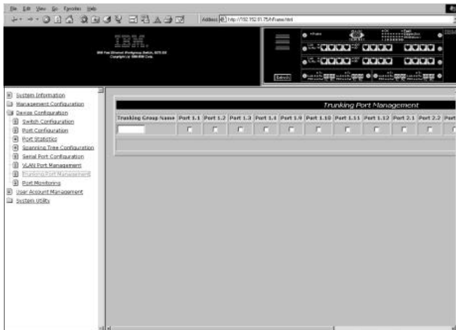
Figure 5-13. Trunking Port Management Panel
