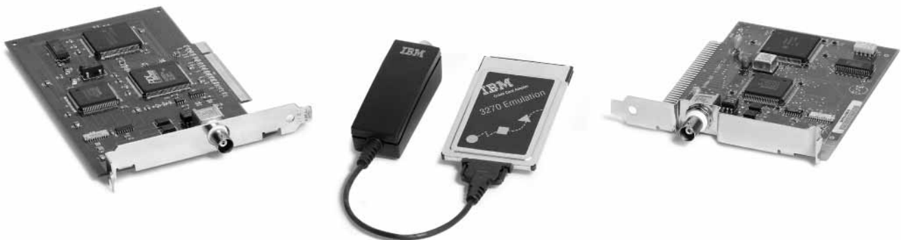
The IBM 3270 Emulation family of adapters: the ISA Adapter, PC Card and cable assembly, and PCI Adapter
