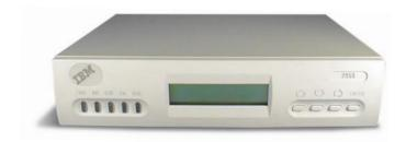
The IBM 7858 Model 336 is a stand-alone modem with Link Problem Determination Aid (LPDA) support for those environments requiring centralized management from a NetView console. It allows your data terminal equipment (DTE) to communicate with other DTEs using a synchronous or asynchronous protocol. The 7858 operates in duplex mode at line speeds of up to 33.6 Kbps over switched and 2-wire or 4-wire leased lines.
