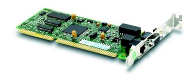
The IBM Turbo 16/4 Token-Ring ISA Adapter is a 16-bit, Plug and Play enabled adapter that features extremely high throughput, memory reduction capabilities and easy installation. This adapter requires as little as 12 KB of DOS memory. The IBM LAN Client allows LAN drivers, protocol stacks and client code to move from conventional and upper memory to extended memory.
