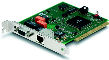
IBM 16/4 Token-Ring PCI Adapter 2 with Wake on LAN
