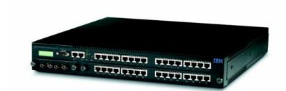
The 8239 Token-Ring Stackable Hub is IBM's newest workgroup offering for the connection and management of devices in a LAN. One to eight hubs can be linked together and managed as one stack, connecting up to 256 devices. The 8239 is a complete replacement for the IBM 8238 Nways® Token-Ring Stackable Hub, offering the latest in Token-Ring technology and advanced network management support. Its attractive design, ease of use and competetive pricing provide real value to Token-Ring users.
