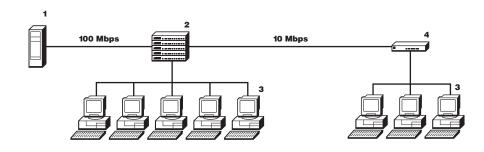
**Solution:** Introduce a 10/100 multi-speed hub into the network providing power users with the bandwidth they require without interfering with users requiring less bandwidth. This configuration allows users to communicate with each other, while protecting the migration of 10-Mbps hubs and the immediate need for power users (at 100 Mbps).
