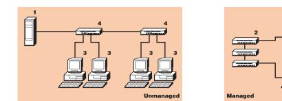
**Solution:** Segment the LAN by connecting power users directly to the 8275-113, offering 10-Mbps Ethernet to the desktop; aggregate 10-Mbps shared hubs to provide additional bandwidth and investment protection. The server or backbone connection gets the high-speed 100-Mbps link, improving network performance.
