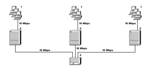
**Solution:** Provide a dedicated, switched 10/100 Ethernet connection to each workstation and server via 8277s.
